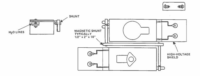
Figure 3. Schematic diagram of a typical chamber layout using two sources
