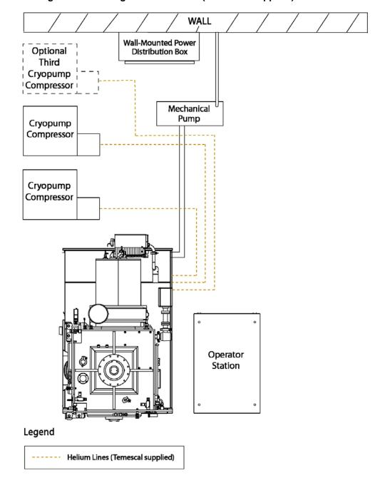
Figure 3-8 Routing of Helium Lines (Temescal Supplied)
